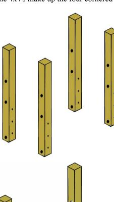
The pipes feed through the bored holes to tie the structure together.
