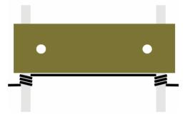
Push a loop of rope up through the bored hole on tread
