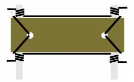
Continue looping and wrapping all 12 treads. Use a clove hitch to secure the rope after the last tread and let the excess rope (there will be plenty) sit on the ground until time to break everything down.
