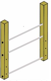
The 3/4 pipe make up the length of the bridge - pipe passes through 4x4 and end caps screwed on.
